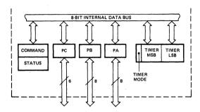
Figure 1. 8155/8156 Internal Registers
